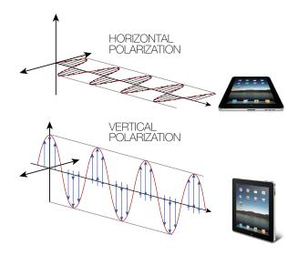
Handheld scanner devices and tablets are constantly moving in horizontal and vertical direction while in use. BeamFlex+ offers thousands of antenna patterns in horizontal and vertical combinations and can maximize the performance of single antenna handheld devices by adapting to the client in real-time.
